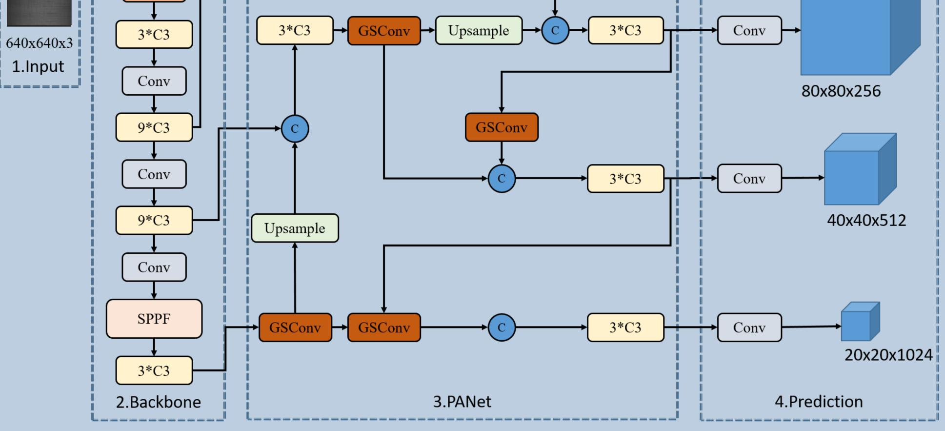
These modules were added to improve the model's performance on glass wool defect detection, with GSConv reducing computation costs while maintaining accuracy, and CBAM enhancing feature representation for small defects in complex backgrounds.
